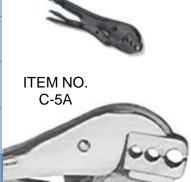
"Hand-Grip" feature permits tremendous pressure. No hammer, vise or other tool needed. Install ferrules and splicers or connection on hose. Offset tool approximately 1/8" from end of ferrule in proper hole and squeeze. Make 1/4 turn and squeeze hard.
