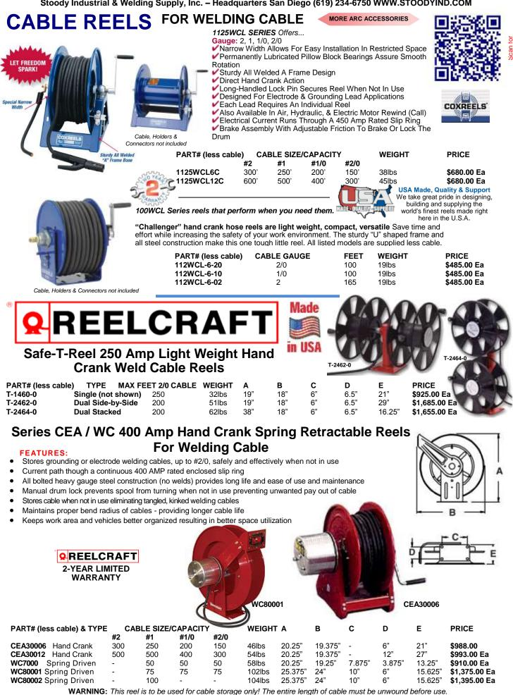
Severe damage to the reel will result if the cable is energized while fully wound on the reel.
