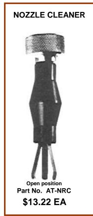
This handy mig nozzle reamer/cleaner uses expanding spring steel blades to quickly remove splatter. By inserting the tool into mig nozzle and turning, you will be assured of unrestricted gas flow and cleaner, stronger welds. There is no need to wait for the nozzle to cool before cleaning. Self adjusting to fit all nozzle sizes.
