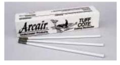
Tuff-Cote tubular steel oxygen-arc cutting electrodes are first coated with an arc stabilizing flux coating, then waterproofed, protecting the flux from moisture absorption and providing electrical insulation.
