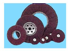
BCR Satin Buffs are constructed of non-woven abrasive material pulled down into a metal clinch ring. This construction allows for great side-to-side flexibility along the work face, making them ideal for operations where they are stacked together with spacers between each section on a pedestal grinder. This creates an inexpensive flexible finishing wheel as wide as you like it!
