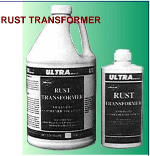
Neutralizes and converts rust to a protective black, glossy, acrylic coating. A combination of acrylic copolymers and acids that will prevent future rusting for up to one year. Dries to a black acrylic/iron coating within 30 minutes. Applied by brush or roller. Nonflammable.
