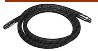
Rubber Air Hose is made from top quality natural rubber compounds and is highly abrasion resistant. This fiber reinforced hose is resistant to the effects of oil, heat 8 ultra-violet light. Pre-cut lengths have solid brass fittings
