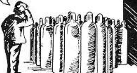
Keep empties from mixing in with the fulls. A quick viewing of your facility and you can find, by the color of the tag, the status of your gas supply.
