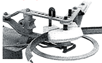
Figure 24-4 Bend Angle Iron 1/2" x 1/2" x 1/8" through 1-1/2" x 1-1/2" x 3/16" to 10" Heel Outward to 14" or larger radius.
