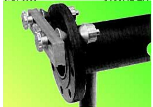
*If adjacent top or bottom holes cannot be used, two-holing can be achieved using side bolt holes. In this instance, the DSL dial is set at 90 degrees and the flange is rotated until the bubble is centered.*
